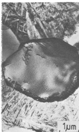
Figure 3 Electron micrograph of the 0% Si alloy after air cooling from 900° C. The microstructure consists of primary \alpha -grains and prior \beta -grains which have been transformed on cooling to a basket-weave \alpha + \beta structure.
